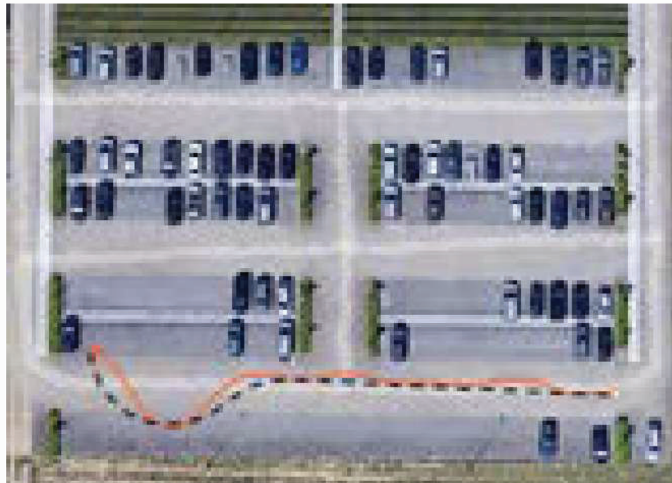
Figure 3: Policy tuned in simulation to reach less than 10cm of tracking accuracy, fails to produce satisfactory performance in real-world
